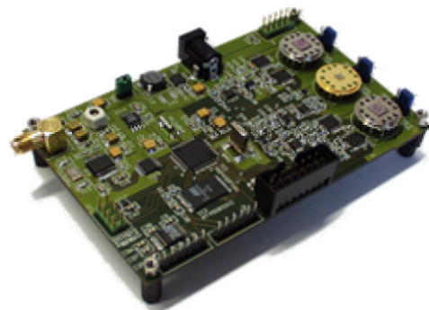
Figure1: The RFID reader with onboard gas sensing capability.
