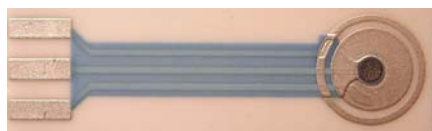
Fig.2. Base substrate with deposited graphite working electrode
