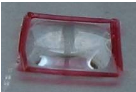
Fig. 2. Glycerol solution deposited on a glass object-plate inside the 3×3 mm drawn square.
