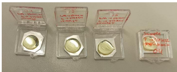
Fig.2. Gold nanoclusters solution incubated on NAA samples.
