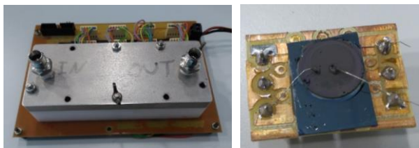
Fig.2. Used test chamber and example of fabricated sensor.
