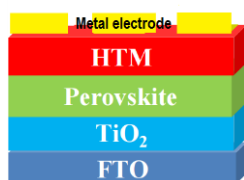
Figure 1: Schematic diagram of perovskite solar cell (PSC).
