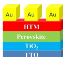
Figure 1: Schematic diagram of perovskite solar cell (PSC).
