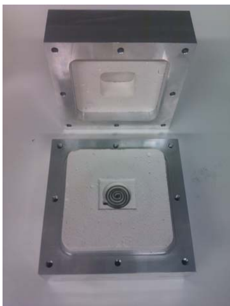
Fig 2. Homemade reactor in which we will produce nanostructures.
